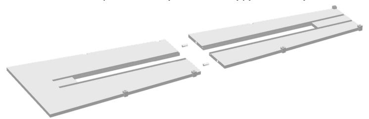
Once these parts have cured, you can add the optional service pit. Turn the foundation over, align the pit and secure with cement. This is a good place to use a drop of CA at each end to hold the pit while the solvent is applied. The pit requires cutting a recess into your platform as the pit hangs about 3/8" below the base. If the pit is not used, you can paint the platform surface dark gray to give the illusion of depth without cutting the recess.
